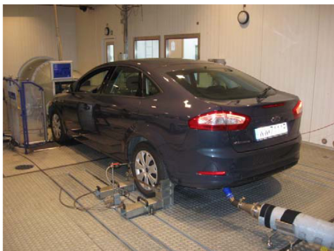
Figure 3. Exhaust emissions laboratory at BOSMAL, showing the chassis dynamometer, windspeed fan, drivers aid and a vehicle connected to the heated Diesel exhaust sampling line, all within the climatic chamber
