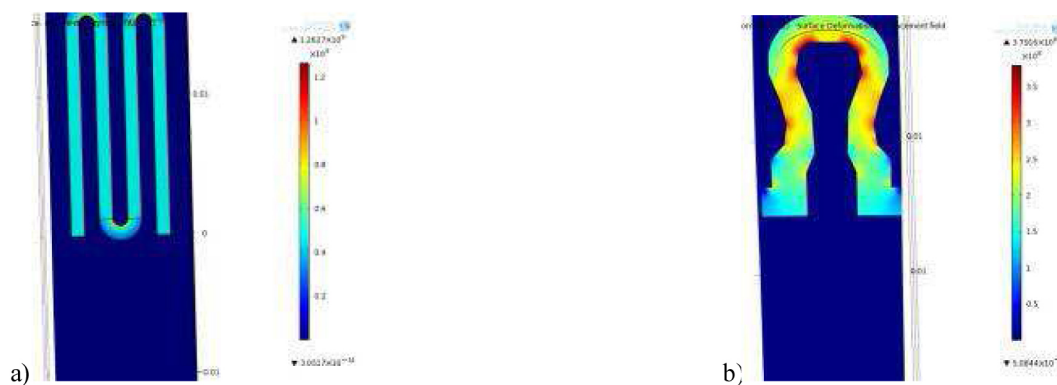
Figure 5. Current density cartography (a) of the “optimized design” and (b) of the “design 1”
