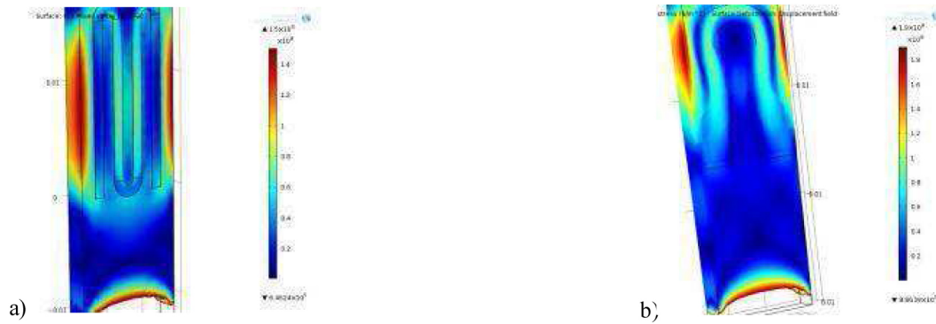
Figure 4. Von Mises stress cartography (a) of the “optimized design” and (b) of the “design 1”
