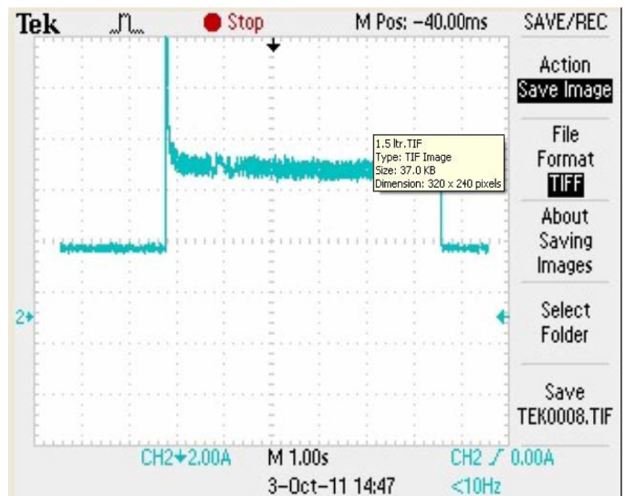
Figure 4. Half Load Condition Washer Motor Operating Current - 2.8 Amps @ 12 Volts
