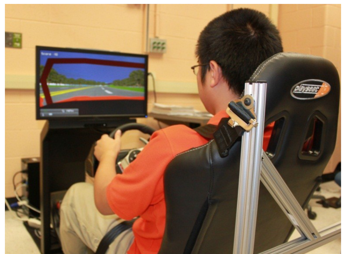
Figure 2. Portable Clemson Automotive Training System (CATS) with seat belt, standard human / vehicle interface, screen display, speaker and the host PC workstation
