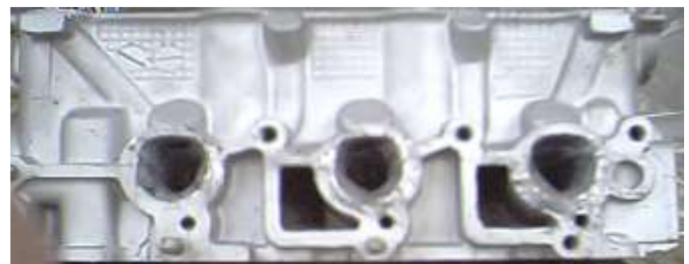
Figure 2. Cylinder head with port modification
