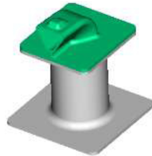
Figure 1. CAD drawing of tri-shape port attached to bore
