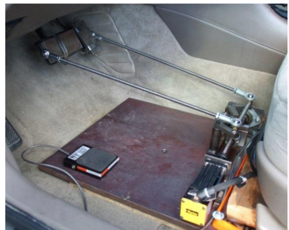
Figure 4. SEA brake and throttle actuator prototype [9]
