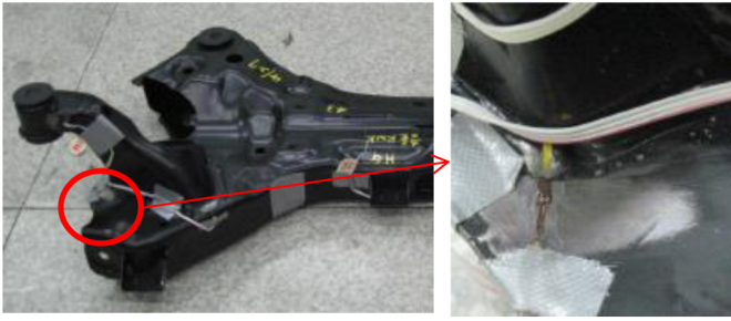
Figure 3. Strain Gage at crack location on bushing mounting front cross member
