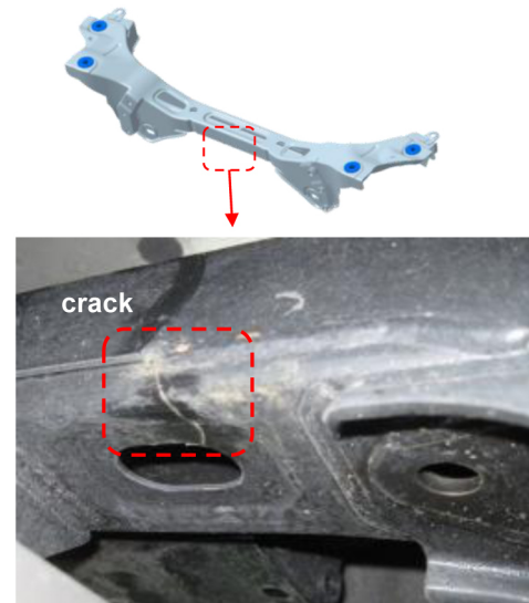
Figure 6. Cracks on bushing mounting rear cross member
