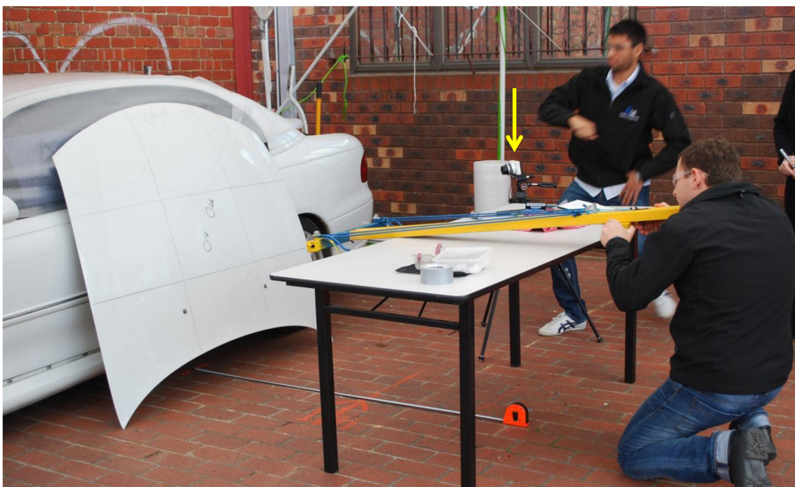
Figure 13. A view of the projectile launching device (yellow). Tape measure on the ground under the table. High speed camera indicated with arrow. In this test, the target body panel was the vehicle's bonnet.
