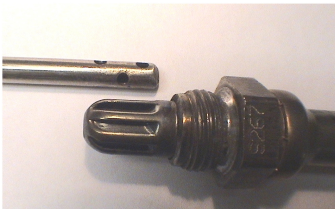
Figure 10. Picture of cross-drilled sample probe and sample PM sensor
