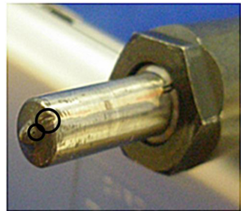
Figure 1. Injector nozzle fitted with miniature thermocouple, the upper circled area contains the thermocouple hot junction and in the lower circle is a nozzle exit hole
