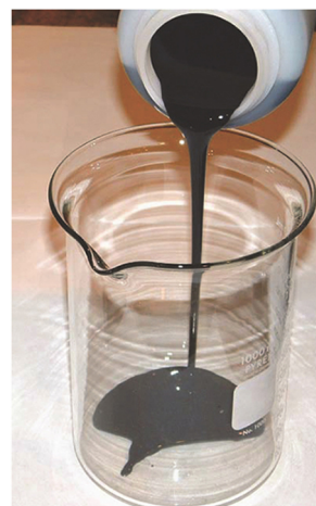
Figure 4. PL pouring into a beaker. PLs are typically dark brown to black in color [28], with a viscosity higher than that of conventional diesel fuel [4,21], and characterized by a smoky odor [26].
