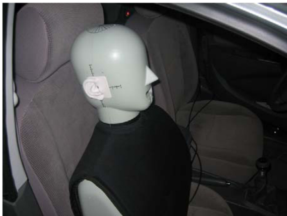
Fig. 1. Artificial head placed at the front passenger seat
