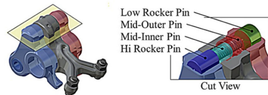
Figure 6. 3-Rocker coaxial synchronizing pin structure
