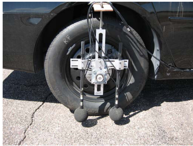
Figure 1. Photograph of dual OBSI probe fixture installed on a test vehicle
