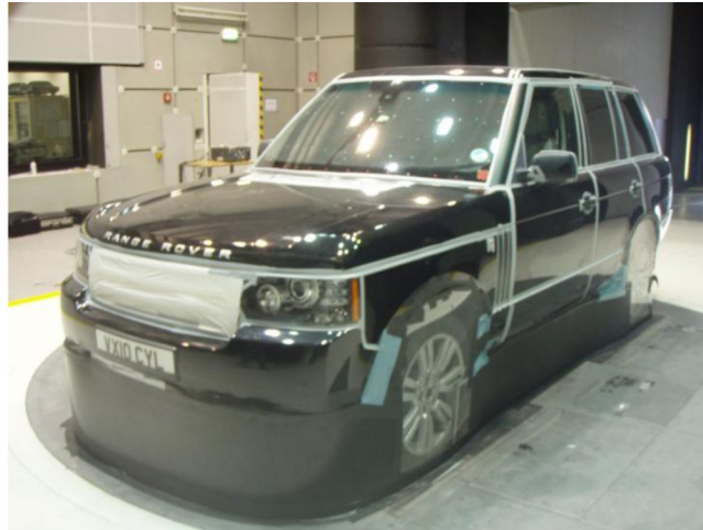
Fig. 1. Standard Test Setup for Vehicle in Acoustic Wind Tunnel with all Seals and Edges Taped and Underbody “Skirt” In Use
