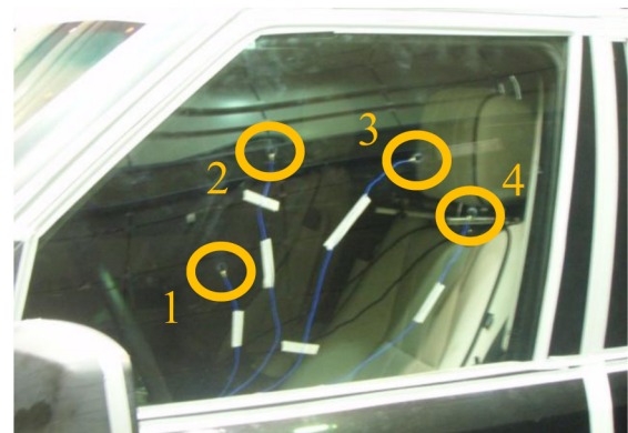
Fig. 4. Lightweight Accelerometer Mounting Positions on Front Side Glass
