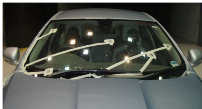
Figure 2. One set of exterior surface microphone locations
