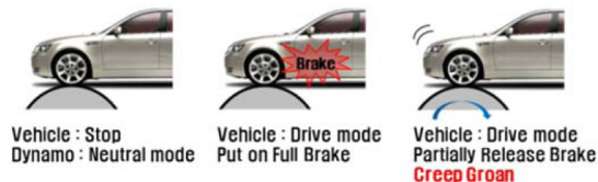
Figure 1. Generating creep groan on chassis dynamometer.
