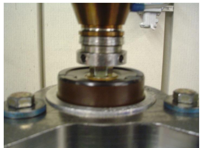
Figure 10. Phenolic Piston Sample fixture into Elastomer Test Machine
