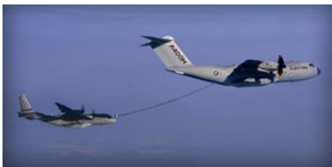
Figure 1. C295 being refueled form an A400M.
