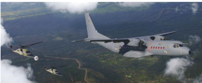
Figure 3. C295 with the AAR kit refueling helicopters
