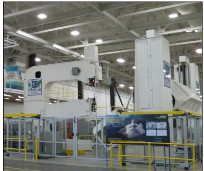
Figure 4.0. Installed CNC Composite Fastening System
