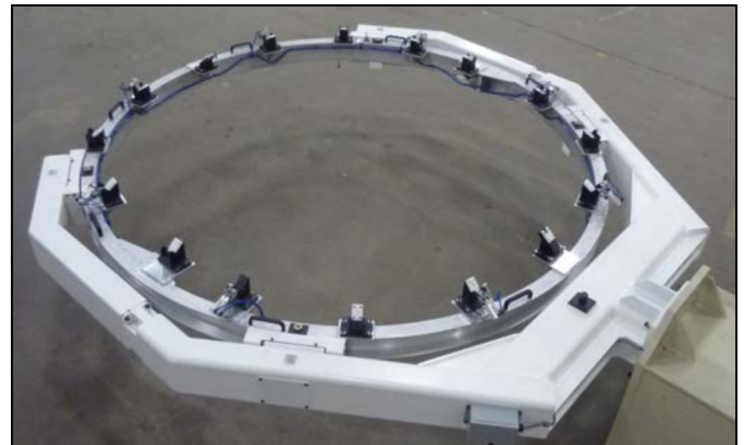
Figure 7.0. Rotating Pneumatic Bulkhead Fixture
