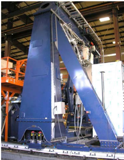
Figure 2. Struts allow more aggressive acceleration and deceleration in the X-direction, reducing cycle time
