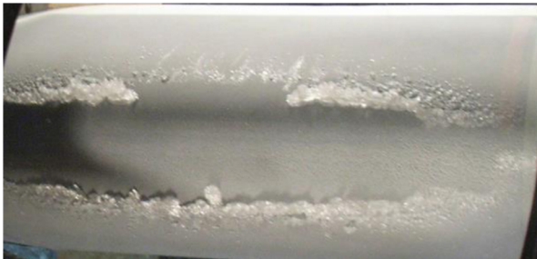
Figure 1. Icing on a superhydrophobically coated test model Airspeed: 90 m/s Ambient temperature: -10 deg. C LWC: 0.42 g/m 3 MVD: 20 microns Duration: 5 min.
