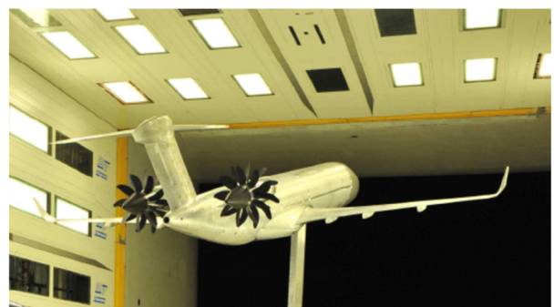
Figure 3. Airbus Z08 A/C rear fuselage pusher CROR wind tunnel model
