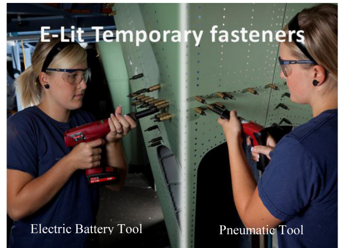
Figure 5. Examples of Temporary fasteners using Desoutter E-LIT and SDP range
