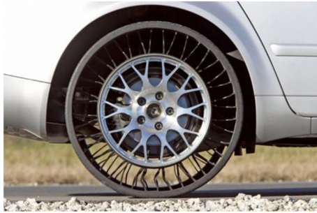
Figure 1. The Michelin® Tweel™, a commercial example of a flexible wheel [5]
