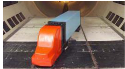
Figure 1. 1/8 scaled GCM geometry in the 12-Ft pressurized wind tunnel [6]
