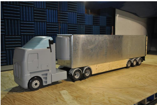
Figure 1. 1:3 scale model in the modified open jet test section.
