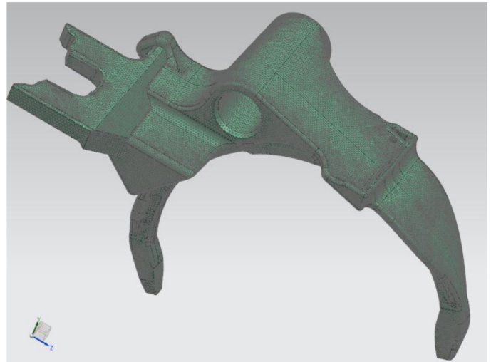
Figure 6. Fine mesh model of Shift Fork.
