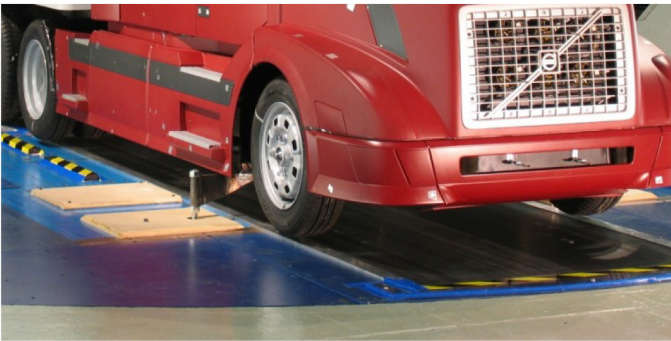
Figure 3. Details of the forward mounts and floor covers.
