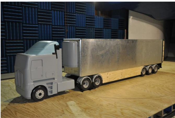
Figure 1. 1:3 scale model in the Monash University 1.4MW wind tunnel.
