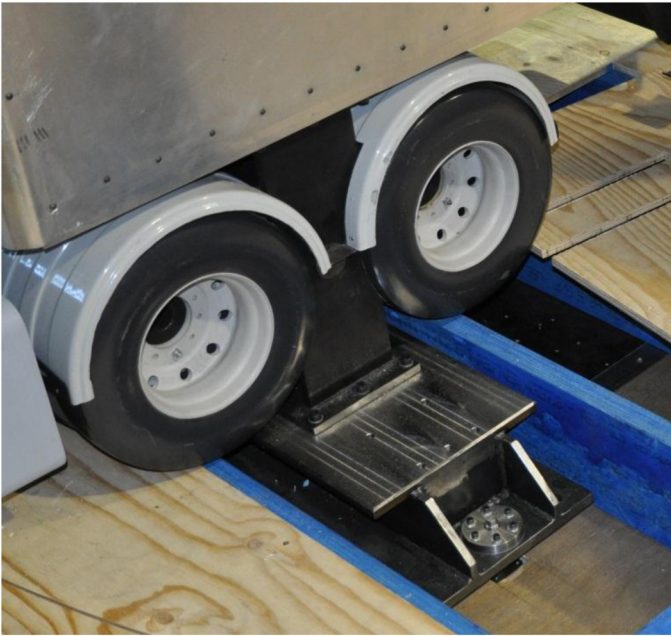
Figure 3. Truck model mounted to force balance beneath the false floor.
