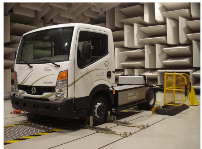
Figure 3. vehicle a hemi-anechoic chamber
