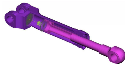
Figure 6. Unlock actuator damping modelling
