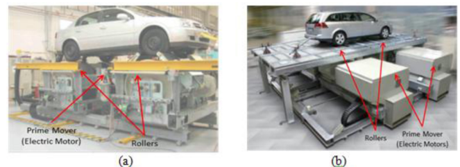
Figure 2. (a) Center Mounted Dynamometer, (b) Inline NVH Dynamometer [3].
