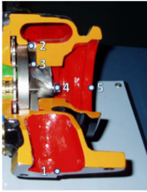
Figure 3. Turbine section and main stations
