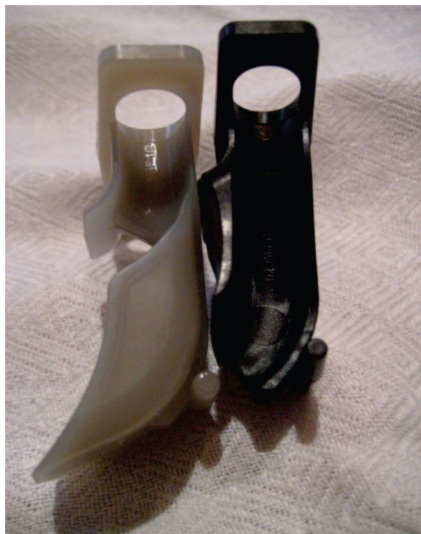
Figure 7. Crank case inserts for different scavenging duct lengths 110mm versus 130mm.
