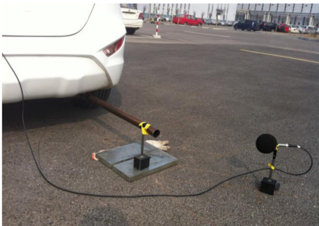
Figure 3. The location of the microphone with respect to the tailpipe exit during the tailpipe noise measurements. This photo shows the case with 700 mm extension.
