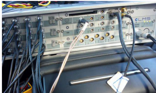
Figure 2. LMS Data acquisition equipment
