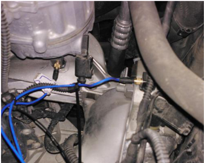
Figure 4. Sensors location on left mount
