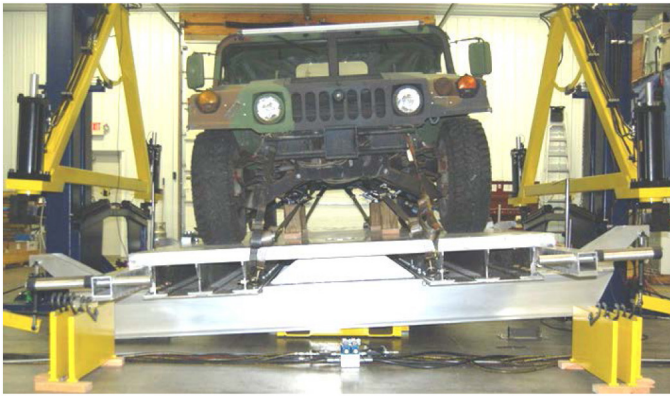
Figure 3. Photograph of short platform supported in roll inertia configuration.
