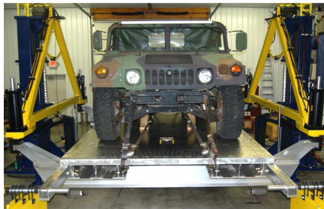
Figure 2. Photograph of short platform supported in pitch inertia/ CG height tests configuration.
