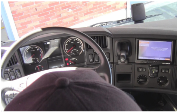
Figure 1. The prototype application for executing remote diagnostic tests. With the in-vehicle display to the right the driver can communicate with the help-desk when tests are executed.
