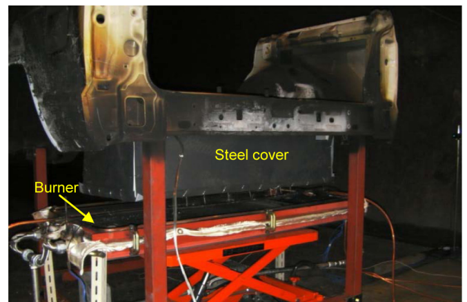
Figure 7. Test 3 setup before burner ignition
