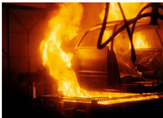
Figure 1. The standard fire exposure test of plastic fuel tanks described in ECE R34, Annex 5 Section 5.0
