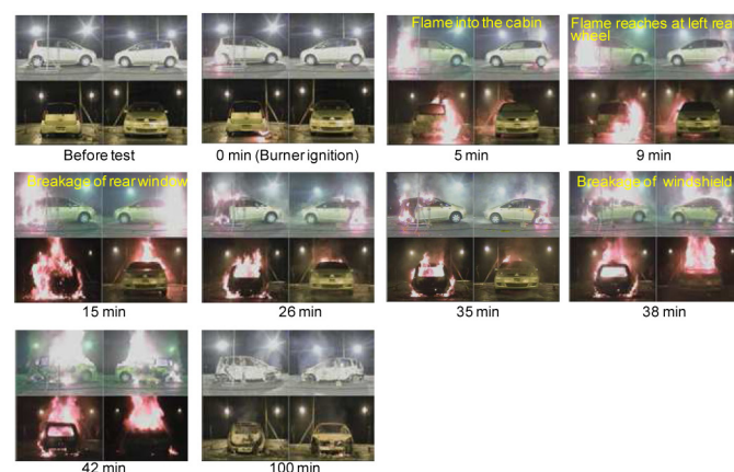
Figure 5. Video images of combustion process by Gasoline Vehicle
