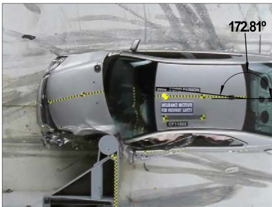
Figure 4. Frame 51, CF11002. 2008 Ford Fusion into 15cm flat steel wall barrier.
