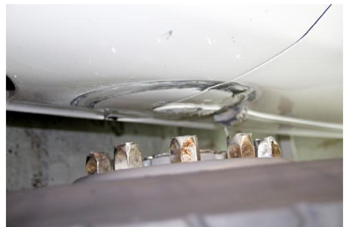
Figure 3. Post-test 4 demonstrating flattening of lug nut cover and corresponding damage to A-hinge pillar.
