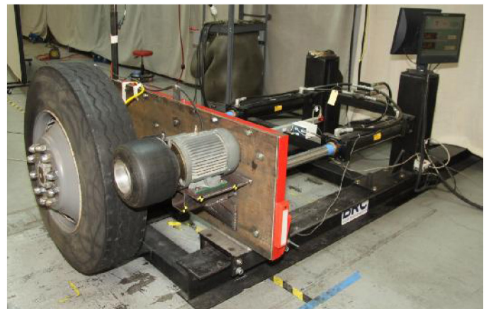
Figure 1. Apparatus used to move spinning tractor tire into passenger vehicles.
