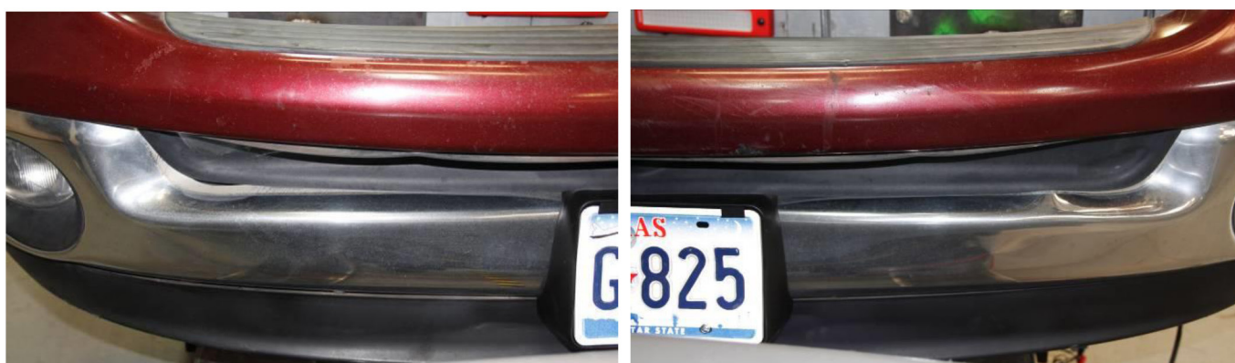
Figure A2.4. Photographs of damage to the front bumper of the Dodge Ram 1500 after test 1Qb.
