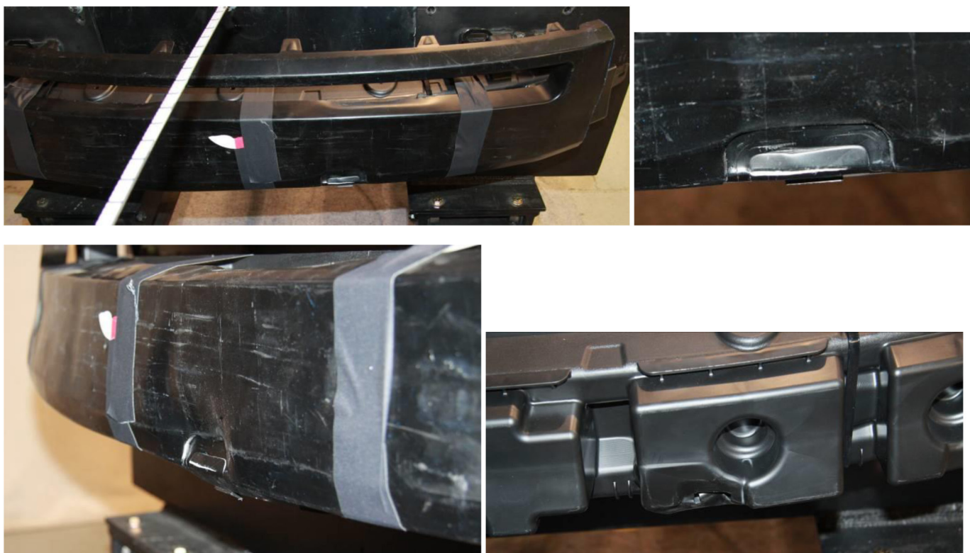
Figure A2.9. Photographs of damage to the front bumper of the Ford Edge after test 2Qa.
