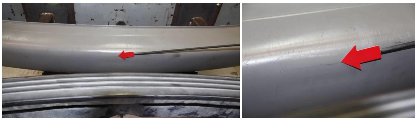
Figure A2.3. Photographs of damage to the rear bumper of Dodge Caravan after test 1Qa.
