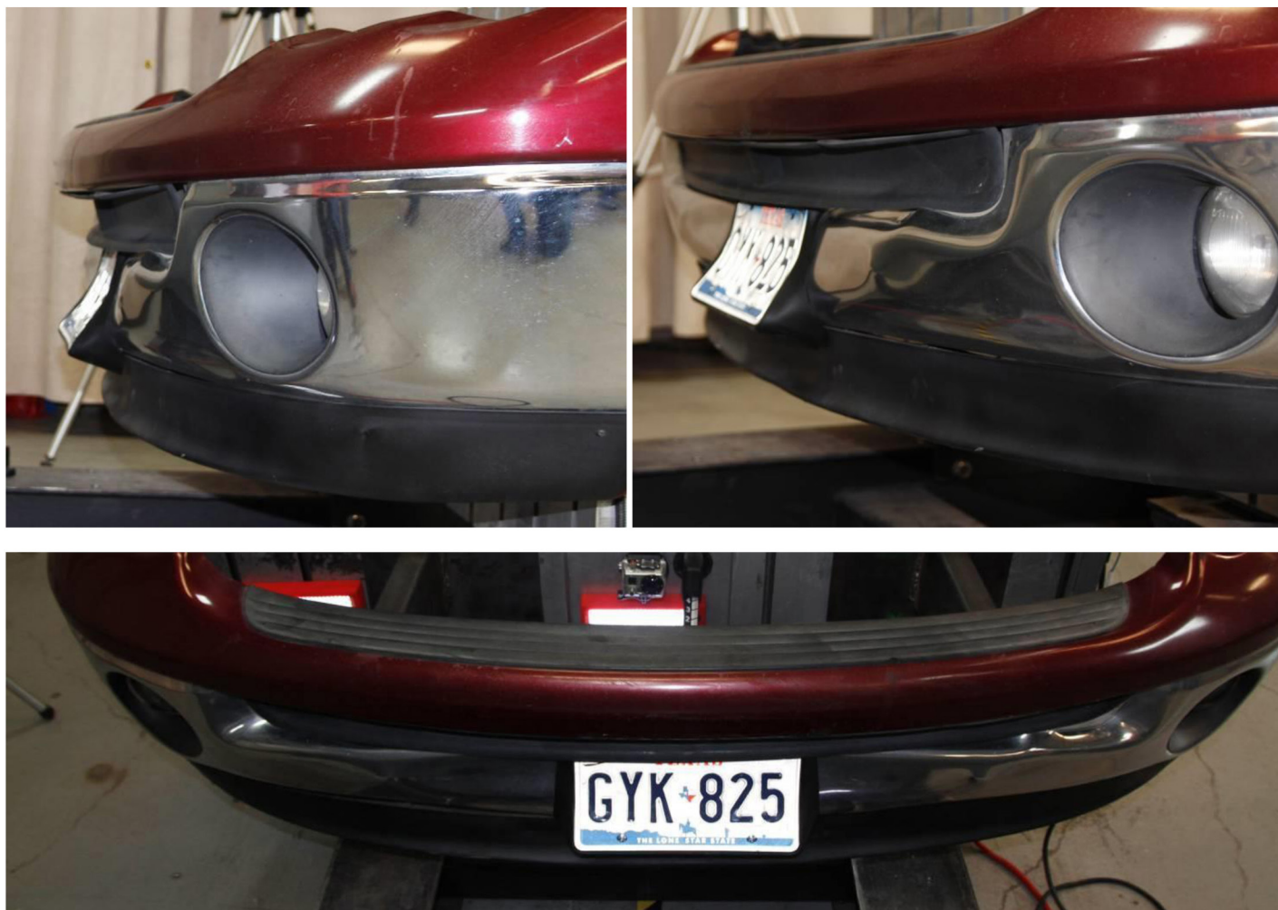
Figure A2.6. Photographs of damage to the front bumper of the Dodge Ram 1500 after test 1Qc.
