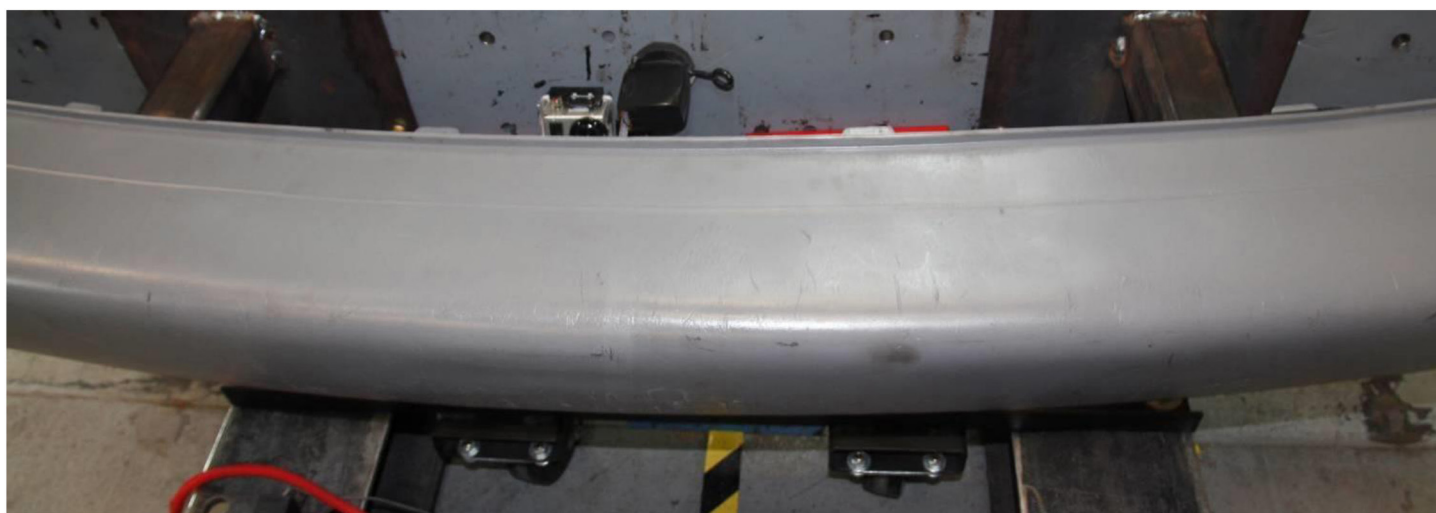
Figure A2.7. Photographs of damage to the rear bumper of Dodge Caravan after test 1Qc.
