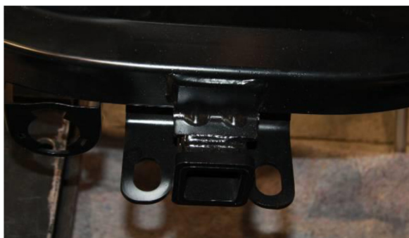
Figure A2.10. Photographs of the undamaged trailer hitch receiver on the rear bumper of the Dodge Nitro after test 2Qa.
