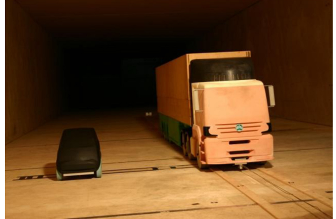
Figure 1. Truck and car model in the wind tunnel.
