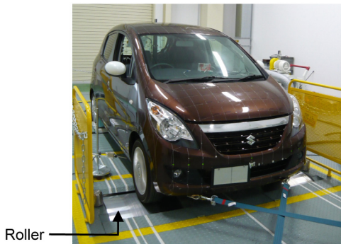
Figure 9. Photograph of chassis dynamometer test
