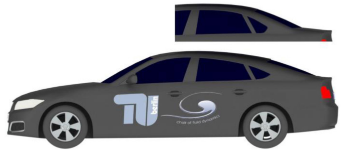
Figure 2. The DrivAer -model with two different rear ends: notchback (top) and fastback (bottom).
