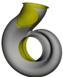
Figure 1. Typical turbine volute geometry in CAD.
