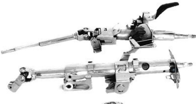
Figure 4. Examples of energy absorbing steering column.
