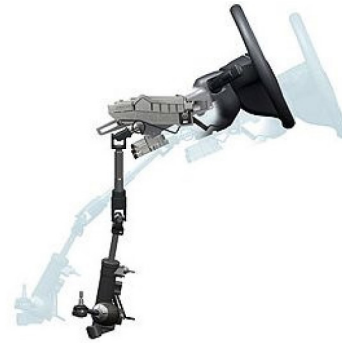
Figure 3. Steering system deformation modes before and after an impact.
